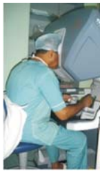
Figure 1 -- A Console where surgeon sits to view surgical field & control the robotic arms, there is place for surgeon to attach his hands & hand motions are translated to surgical instruments, it has 3DViewer.
