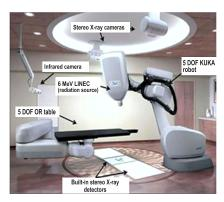
The Cyberknife was invented by Dr. John Adler, a neurosurgeon in Stanford, USA, during the 1990s. Its robotic arm has 6 degrees of freedom of movement, unlike the conventional linear accelerator, which has only rotational movement in one plane. The treatments are non-isocentric, making it possible for the beams to be directed from any desired angle.
